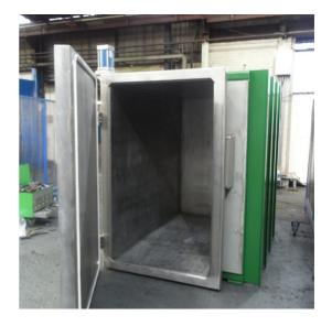
The door and front end of the chamber can be located inside a High Care Area, whilst the external rear of the chamber can be positioned through a dividing wall in a non-food plant area.
